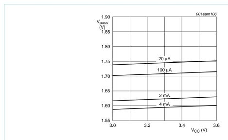
Fig 11. Pass voltage versus supply voltage;  $T_{amb} = -40$  °C (typical)
