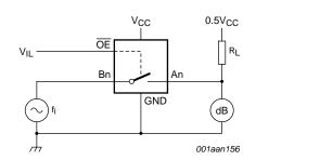
Adjust  $f_i$  voltage to obtain 0 dBm level at output. Increase  $f_i$  frequency until dB meter reads -3 dB.
